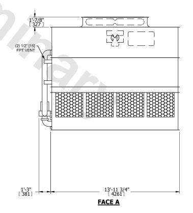
DRAWN BY: NO. OF SHIPPING SECTIONS **SHIPPING** OPERATING HEAVIEST SECTION 13040 lbs+ [5915] kg+ 20100 lbs+ [9120] kg+ 11050 lbs+ [5015] kg+ WEIGHT WEIGHT WEIGHT
