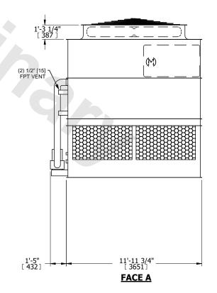
DRAWN BY: SLR NO. OF SHIPPING SECTIONS **SHIPPING OPERATING** HEAVIEST SECTION 12390 lbs+ [5625] kg+ 19900 lbs+ [9030] kg+ 9840 lbs+ [4465] kg+ WEIGHT WEIGHT WEIGHT
