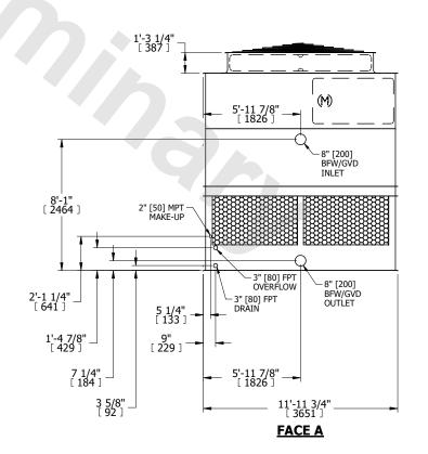
DRAWN BY: JLG NO. OF SHIPPING SECTIONS **SHIPPING** OPERATING HEAVIEST SECTION 6620 lbs+ [3005] kg+ 11580 lbs+ [5255] kg+ 4200 lbs+ [1910] kg+ WEIGHT WEIGHT WEIGHT
