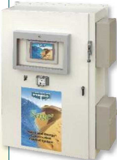
The EVAPCO eco-ATWB closed circuit coolers utilize the optional Sage<sup>2</sup>™ water and energy conservation control system which controls Dry & Evaporative modes of operation. The control system operates by measuring and analyzing water inlet and outlet temperature simultaneous with ambient dry bulb monitoring in order to minimize the evaporative cooling mode of operation and to save system water. The Sage can also be programmed to operate with a water savings or energy savings priority.
