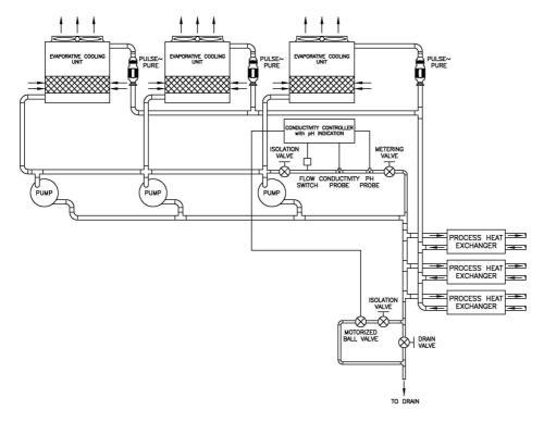
Figure 14 General field installed arrangement showing multiple evaporative cooling units each with a dedicated *Pulse*~Pure<sup>™</sup> system.
