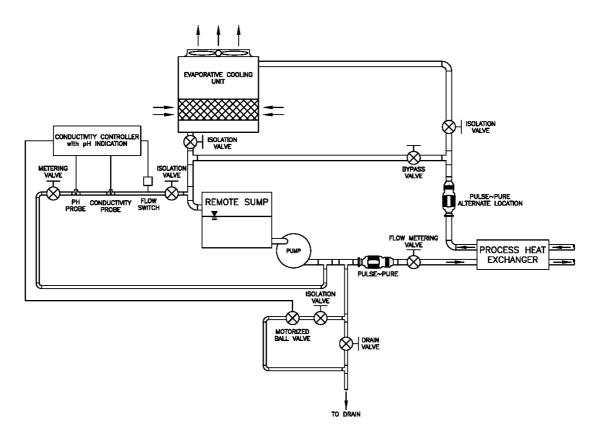
Figure 12 General field installed arrangement of the *Pulse*~Pure<sup>™</sup> system in a system with a single evaporative cooling unit with remote sump.
