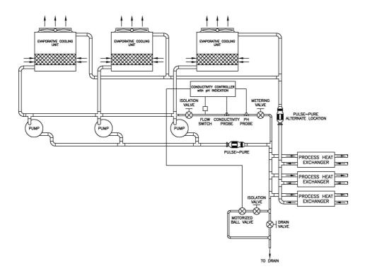
Figure 13 General field installed arrangement of a single *Pulse*~Pure<sup>™</sup> system in a system with multiple evaporative cooling units.
