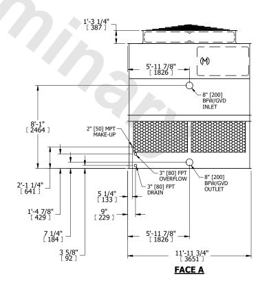
SHIPPING WEIGHT 11580 lbs+ [5255] kg+ HEAVIEST SECTION WEIGHT 4200 lbs+ [1910] kg+ NO. OF SHIPPING SECTIONS 2 DRAWN BY: JLG
