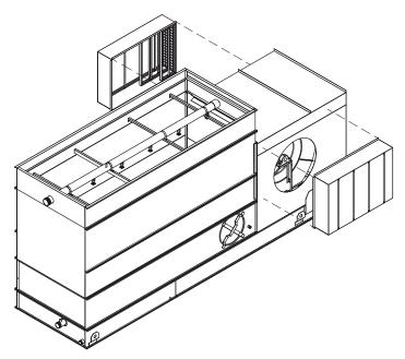
Figure 10 – Rigging Fan-Side Sound Attenuator Assembly
