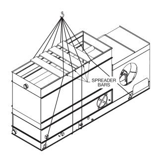
Figure 3b – Alternative Safety Sling Rigging
