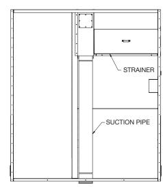
Figure 12a – Strainer Location on 3' (1 m) and 5' (1.5 m) Wide Units
