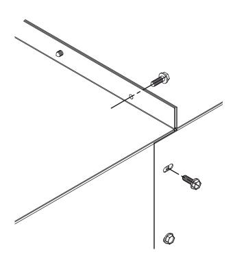
Figure 9 - Fan-End Sound Attenuator Assembly Details
