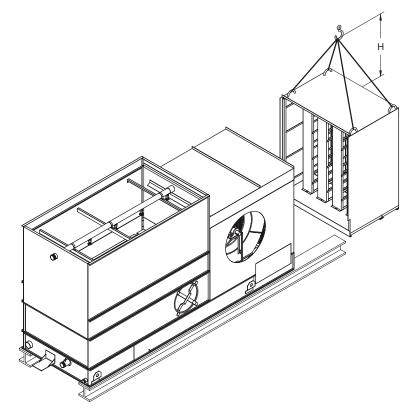
Figure 8 – Rigging Fan-End Sound Attenuator Assembly
