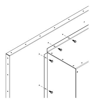
Figure 11 – Fan-Side Sound Attenuator Assembly Details
