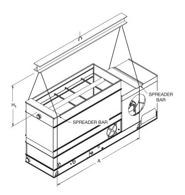
Figure 2a – Recommended Rigging - LP/LR Main Unit
