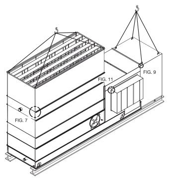
Figure 5 – Discharge and Intake Accessory Rigging
