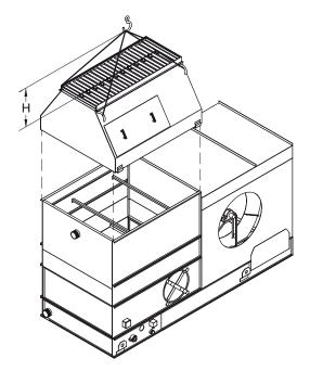
Figure 6a – Rigging Straight Discharge Hood or Discharge Attenuation
