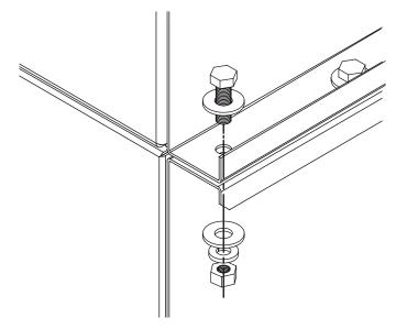
Figure 7 – Discharge Hood or Attenuation Assembly Details
