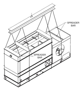
Figure 3a - Recommended Safety Sling Rigging
