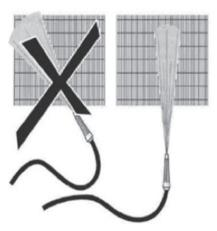
Figure 16 – Always Clean Fins in Vertical Direction
