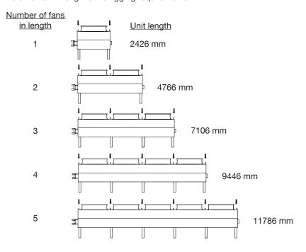
Figure 10 - Lifting Ear Requirements for 2340 mm Incremental Fin Length
