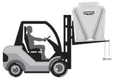
Figure 12 - V Coil Unit Forklift Lifting Requirements
