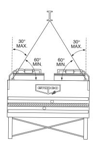
Figure 5 - Minimum Crane Lifting Angles
