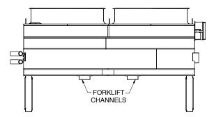
Figure 3 - Flat Coil Forklift Channel Locations
