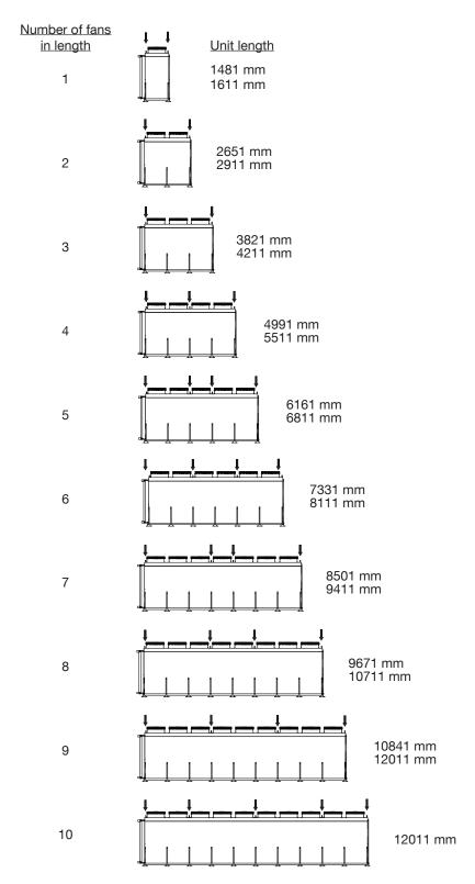
Figure 15 – Lifting Ear Requirement for 1170 mm and 1300 mm Incremental Fin Lengths
