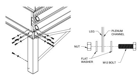
Figure 2 - Flat Unit Leg Attachement
