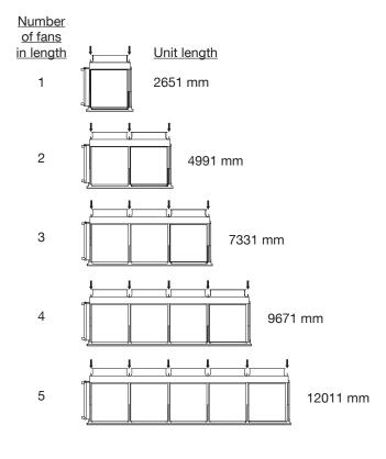
Figure 17 – Lifting Ear Requirement for 2340 mm Incremental Fin Lengths
