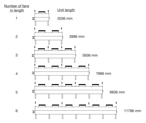
Figure 7 - Lifting Ear Requirements for 1950 mm Incremental Fin Length
