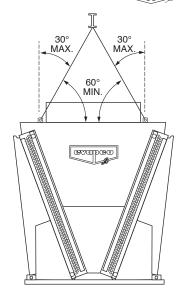
Figure 13 - Minimum Crane Lifting Angles
