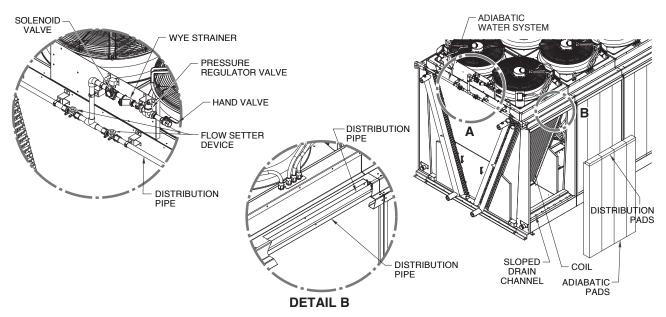
Figure 17 - Adiabatic Air Pre-Cooling System Components
