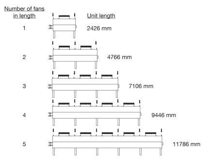
Figure 8 – Lifting Ear Requirements for 2340 mm Incremental Fin Length
