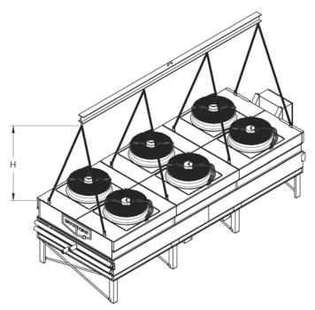
Figure 6 - Rigging Beam Height Requirements
