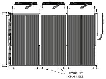
Figure 11 - V Coil Forklift Channel Locations
