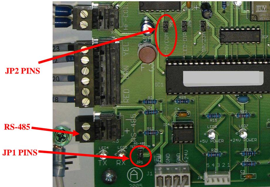
**Figure 8** User connections in the Pulse Panel for monitoring and control using RS-485 protocol.
