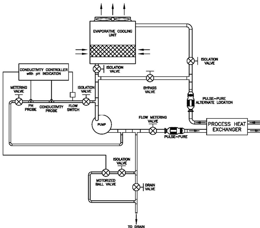
**Figure 11** General field installed arrangement of the *Pulse~Pure*<sup>™</sup> system in a system with a single evaporative cooling unit with integral basin.
