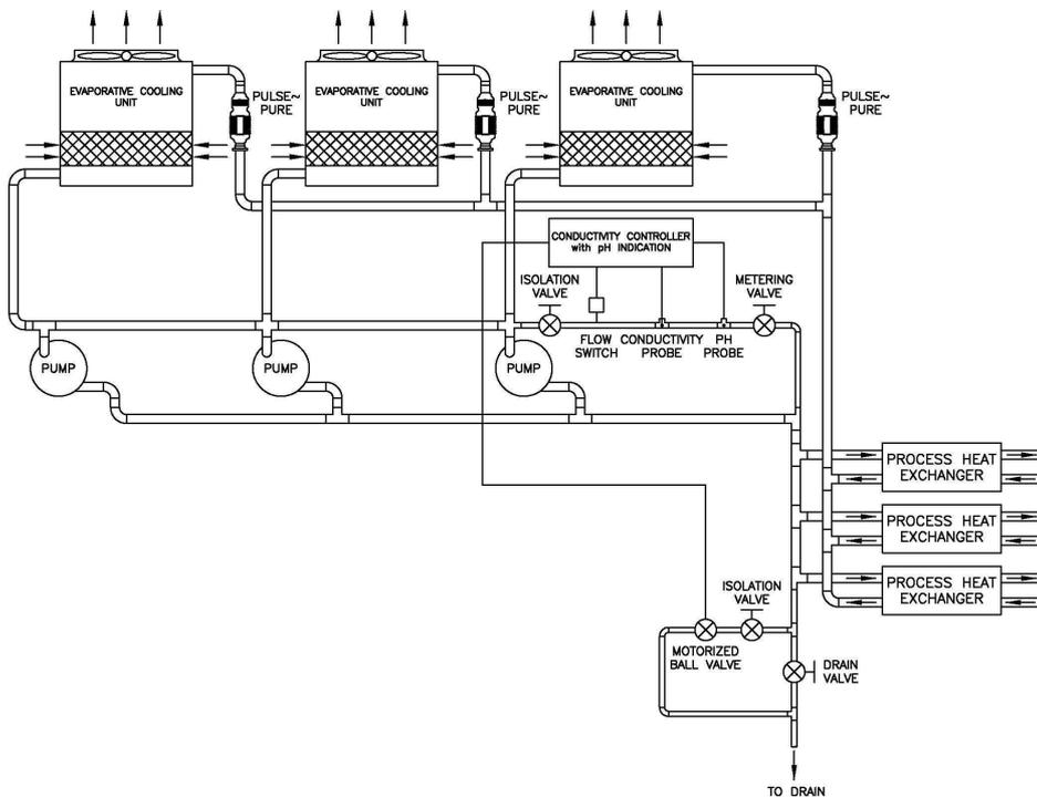
Figure 14 General field installed arrangement showing multiple evaporative cooling units each with a dedicated *Pulse~Pure™* system.
