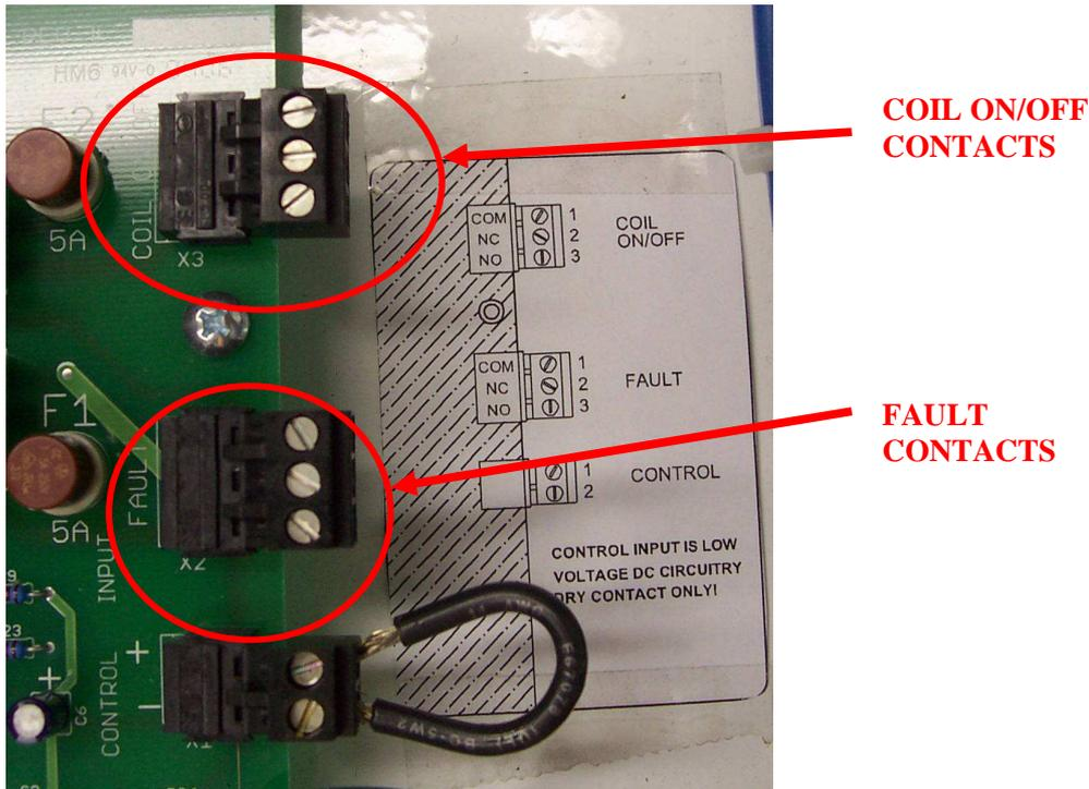
Figure 9 User connections in the Pulse Panel for monitoring coil operation and fault conditions.
