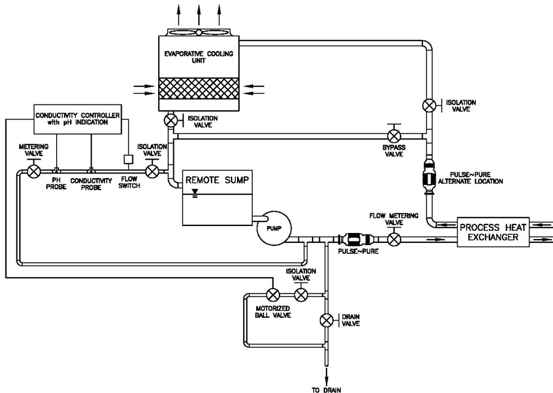
**Figure 12** General field installed arrangement of the *Pulse~Pure*<sup>™</sup> system in a system with a single evaporative cooling unit with remote sump.
