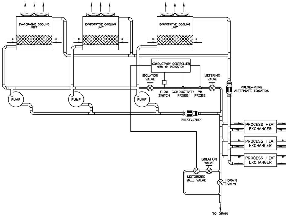
Figure 13 General field installed arrangement of a single *Pulse~Pure™* system in a system with multiple evaporative cooling units.
