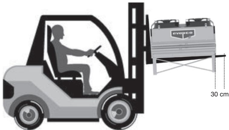
**Figure 4 – Flat Coil Units Forklift Lifting Requirements**
