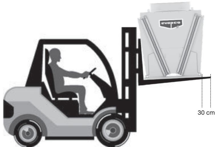
**Figure 12 – V Coil Unit Forklift Lifting Requirements**
