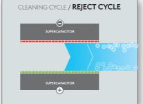
Supercapacitors reverse polarity to reject ions to drain at reduced flow rate
