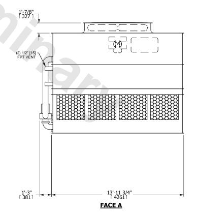
DRAWN BY: SLR NO. OF SHIPPING SECTIONS **SHIPPING** OPERATING HEAVIEST SECTION 11150 lbs+ [5060] kg+ 17540 lbs+ [7960] kg+ 9160 lbs+ [4155] kg+ WEIGHT WEIGHT WEIGHT
