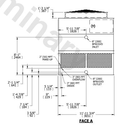
SHIPPING WEIGHT 6620 lbs+ [3005] kg+ OPERATING WEIGHT 11580 lbs+ [5255] kg+ HEAVIEST SECTION WEIGHT 4200 lbs+ [1910] kg+ NO. OF SHIPPING SECTIONS 2 DRAWN BY: JLG
