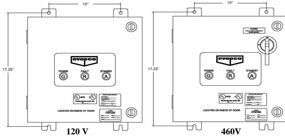
**Figure 15 120 V (left) and 460 V (right) Pulse Panels.**
